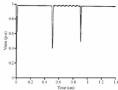
Figure. 10 Alleviated voltage sag at load point with DVR
