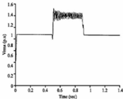
Figure. 7 Voltage Swell at load point without DSTATCOM
