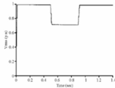
Figure. 9 Voltage sag at load point without DVR
