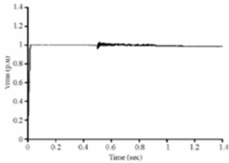
Figure. 12 Alleviated Voltage swell in RMS at load point with DVR
