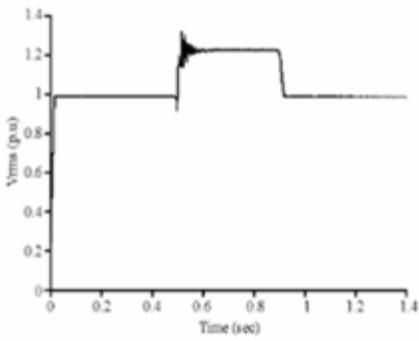
Figure. 11 Voltage Swell in RMS at load point without DVR
