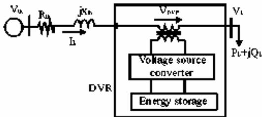
Figure. 2 Schematic diagram of Dynamic Voltage Restorer
