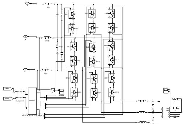
Figure. 14 Matrix converter arrangements which is used in the implementation of UPFC
