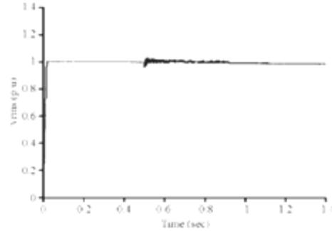
Figure. 8 Alleviated voltage swell at load point with DSTATCOM
