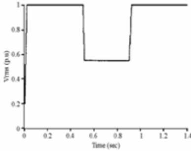
Figure. 5 Uncompensated RMS Voltage at load point without DSTATCOM
