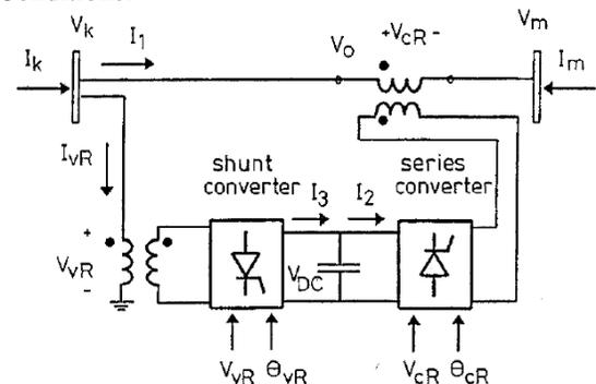
Figure. 4 Schematic diagram of Unified Power Flow Controller
