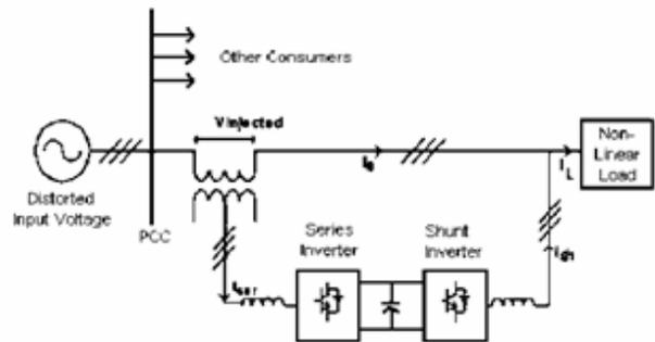
Figure. 3 Schematic diagram of Unified Power Quality Conditioner
