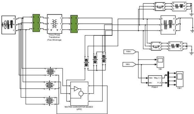
Figure. 13 Closed loop control of Matrix Converter based UPFC
