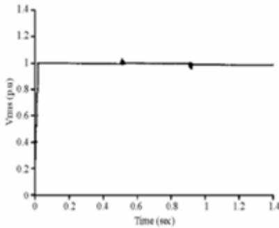
Figure. 6 Compensated Voltage RMS at load point with DSTATCOM
