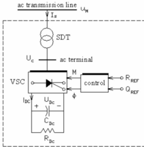
Figure. 1 Schematic diagram of Distribution Static Synchronous Compensator
