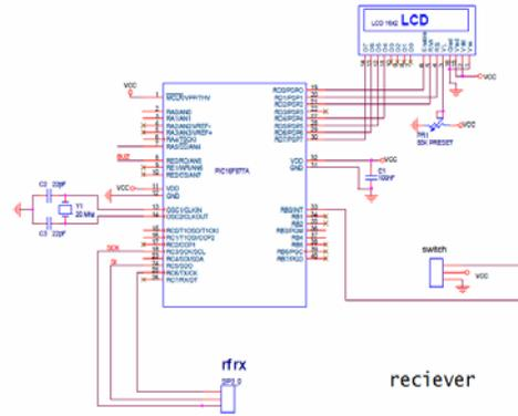
Figure 4.3 Circuit Diagram of Receiver
