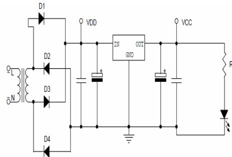
**Figure 4.1** Circuit Diagram of Power supply
