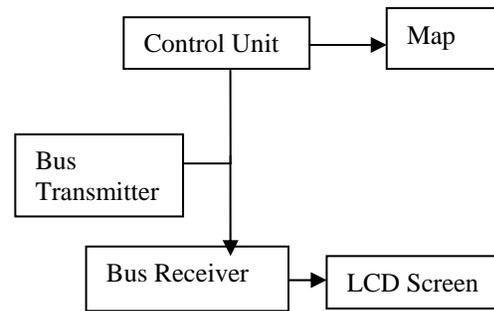
**Figure 3.1** functional block diagram of Real Time Bus Monitoring and Passenger Information System.
