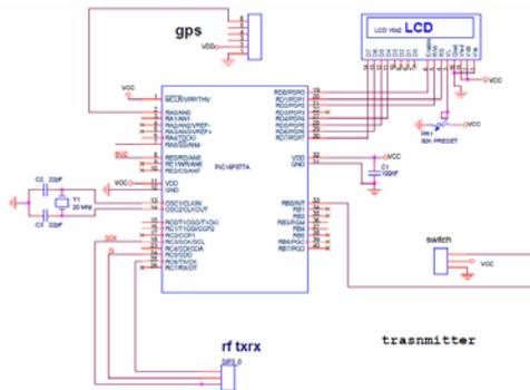
Figure 4.2 Circuit Diagram of Transmitter
