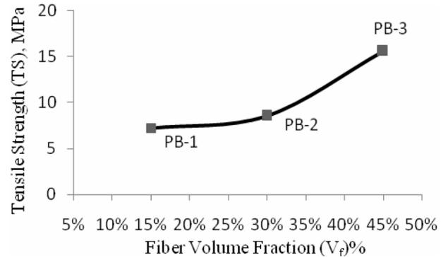
Fig: 6 Variation of tensile strength with respect to the fiber volume fraction
