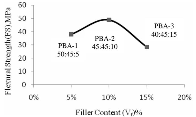
Fig: 9 Variation of flexural strength with respect to the filler content
