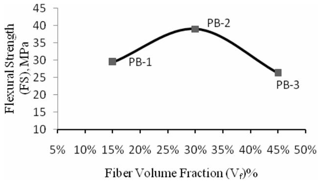
Fig: 7 Variation of flexural strength with respect to the fiber volume fraction
