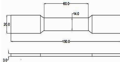
Fig: 2 Specifications of Tension test specimen
