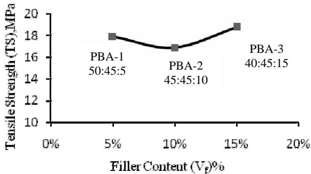
Fig: 8 Variation of tensile strength with respect to the filler content
