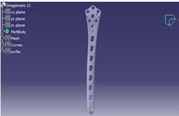
Fig 7 Surface model of locking plate
