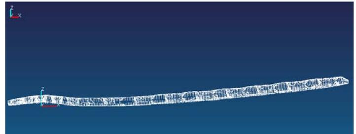
Fig 4 Point Cloud data of Locking Plate
