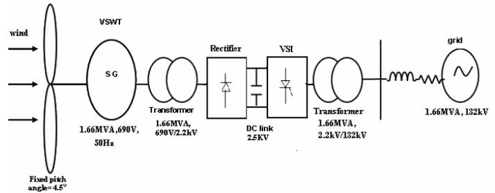
Figure 1. Schematic diagram of modeled VSWT with DDSG
