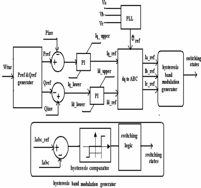
Figure 4. Hysteresis band current control scheme of VSC
