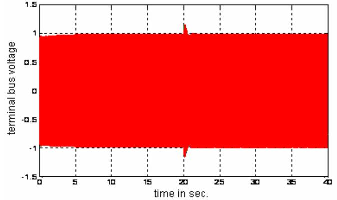
Figure 13. Phase voltage in p.u in grid side of VSWT with DDSG
