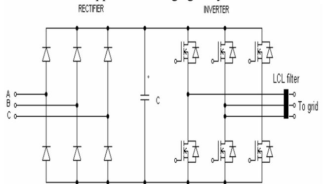
Figure 3. Rectifier and VSC circuit for VSWT modeling
