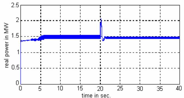
Figure 9. Real power output (1.5MW) of VSWT with DDSG
