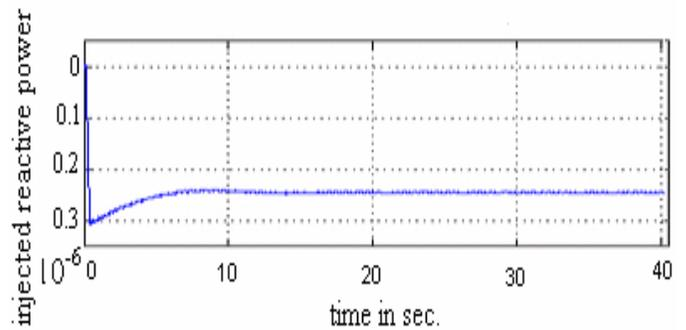
Figure 15. Injected reactive power 0.25MVAR in grid side of VSWT with DDSG
