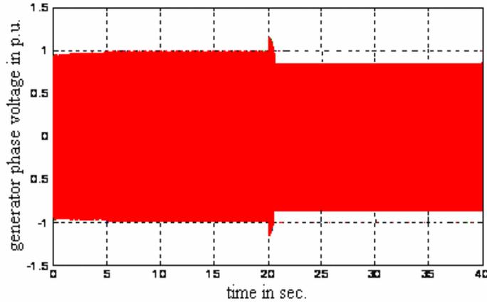
Figure 11. Generated phase voltage in p.u. (690V) of VSWT with DDSG
