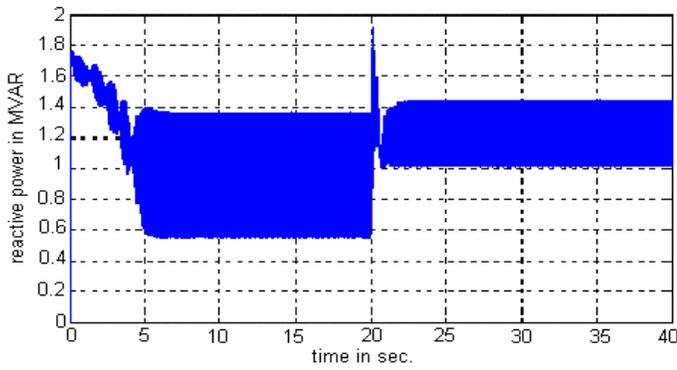
Figure 10. Reactive power generated by VSWT with DDSG
