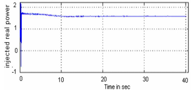
Figure 14. Injected real power 1.5MW in grid side of VSWT with DDSG
