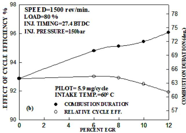
Figure 14. Effect of EGR on Relative Cycle Efficiency and Combustion Duration
