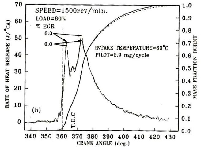
**Figure 3. Effect of Hot EGR on Heat Release Rate and Mass Fraction Burnt**
