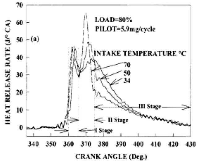
**Figure 1. Combustion Stages in LPG + Diesel Dual Fuel Engine**
