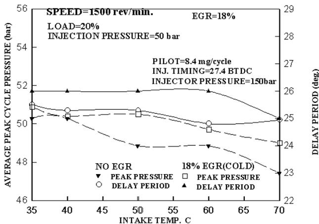
Figure 11. Effect of Intake Temperature on Peak Cycle Pressure and Delay Period
