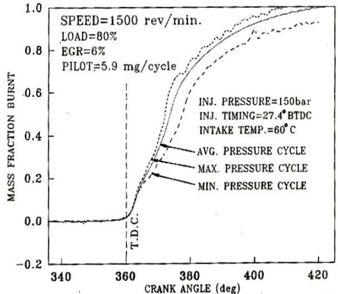
**Figure 4. Crank Angle vs. Mass Fraction Burnt of Three Cycles**
