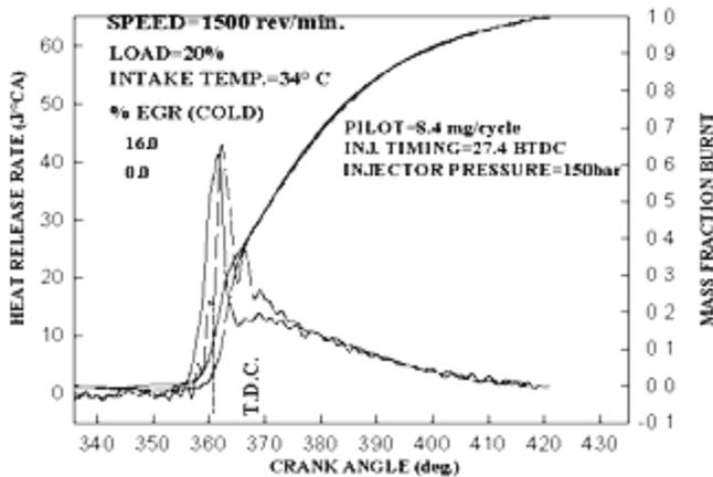
**Figure 5. Effect of Cold EGR on Heat Release Rate and Mass Fraction Burnt**
