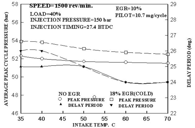
Figure 12. Effect of Intake Temperature on Peak Cycle Pressure and Delay Period
