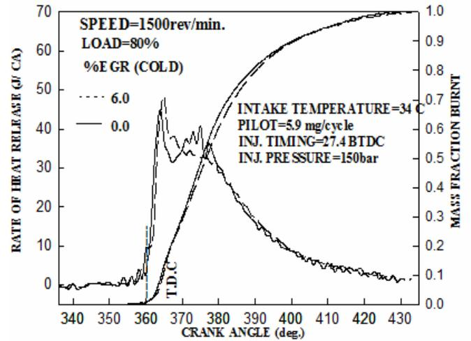
**Figure 6. Effect of Cold EGR on Heat Release Rate and Mass Fraction Burnt**
