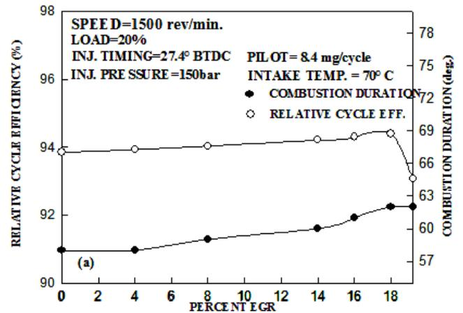
Figure 13. Effect of EGR on Relative Cycle Efficiency and Combustion Duration
