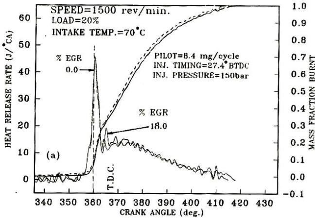
**Figure 2. Effect of Hot EGR on Heat Release Rate and Mass Fraction Burnt**
