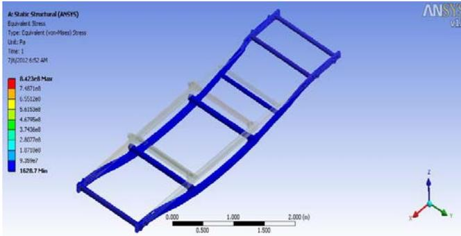
Fig: expandable chassis
