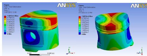
Figure 2: Comparison between total deformation
