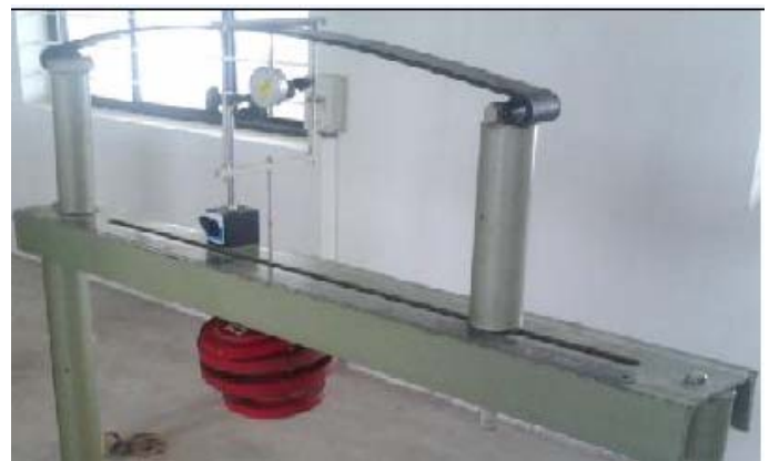
Fig.1.Leaf spring deflection test rig.
