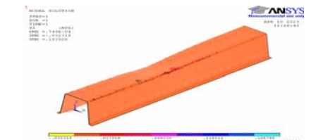
Fig. 10 Stress after applying 17.658 N force at nodal point
