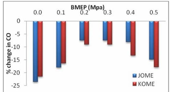
Figure 6. Percentage change of CO Emission with Diesel Fuel
