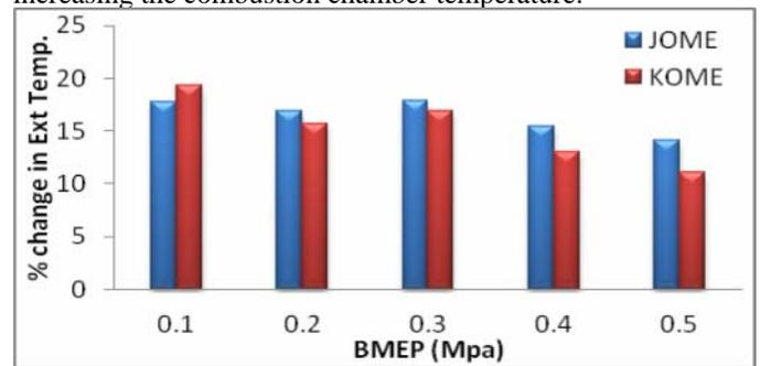
Figure 5. Percentage change of Exhaust gas Temperature with Diesel Fuel
