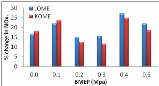
Figure 8. Percentage change of NOx Emission with Diesel Fuel
