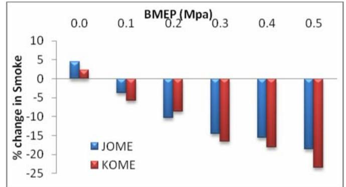
Figure 9. Percentage change of Smoke Emission with Diesel Fuel
