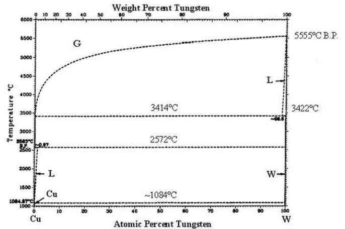
**Fig. 2:** Equilibrium Phase Diagram of the W-Cu System at 1 atm.
