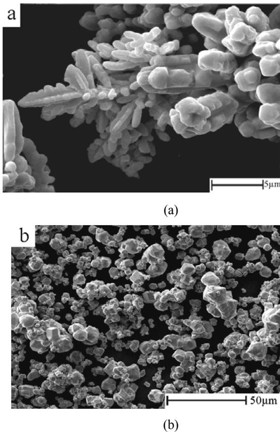
**Fig. 1:** Morphology of (a) pure Copper and (b) Tungsten powder
