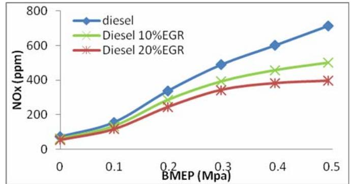
Figure 6. Variation of NOx Emission with the BMEP
