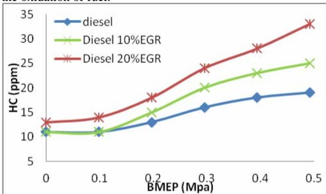
Figure 5. Variation of HC Emission with the BMEP
