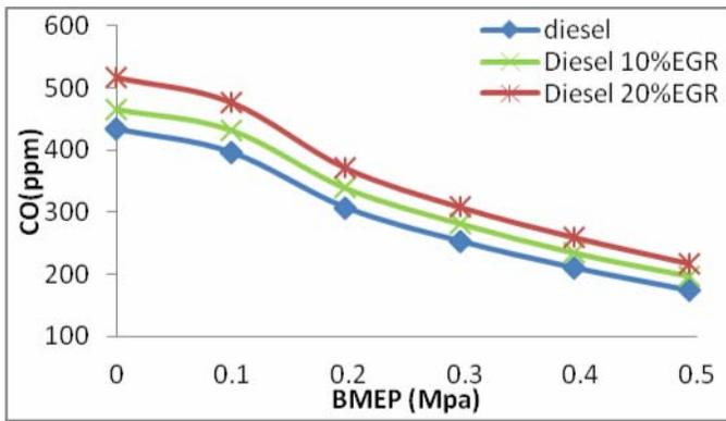
Figure 4. Variation of CO Emission with the BMEP
