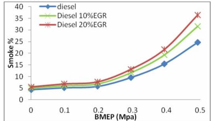
Figure 7. Variation of Smoke Emission with the BMEP
