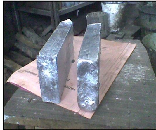
Figure 1: (a) As cast A356 Al-alloy
