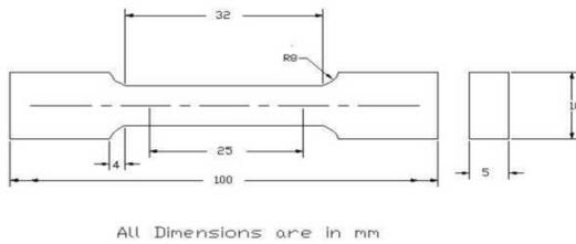
Figure 3 Flat tensile Test Specimen
