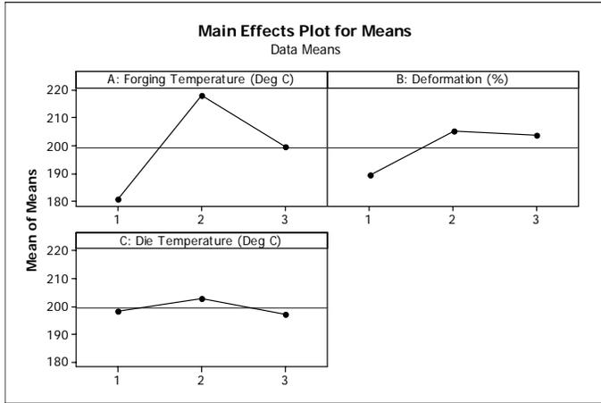
Figure 4 Main Effect Plot for Tensile Strength
