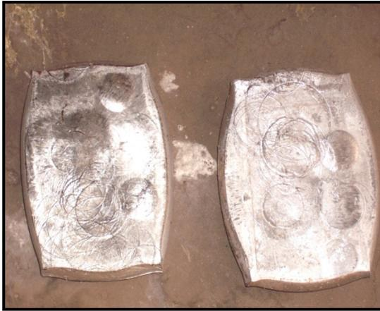
Figure 2: (b) Semi-solid Forged Samples
