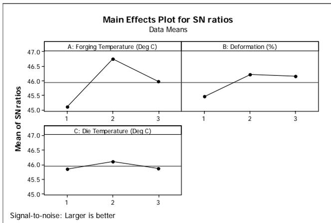
Figure 5 Mean S/N Ratio Plot for Tensile Strength
