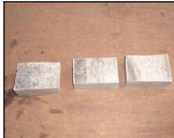
Figure 1: (b) Sample of A356 for Semi-Solid Forging
