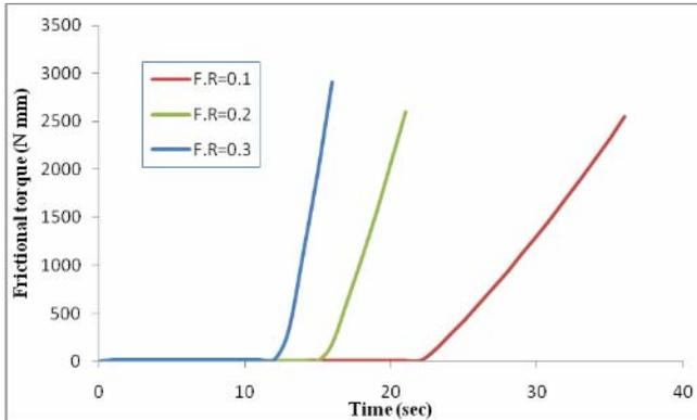
Fig. 3 Effect of Friction coefficient on Frictional torque
