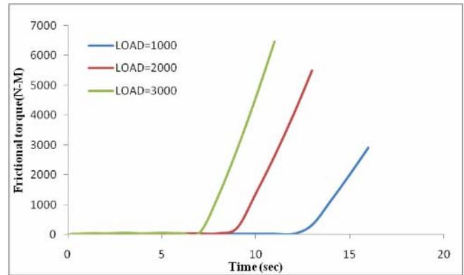
Fig. 7 Effect of Load on frictional torque
