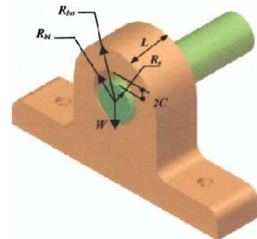
Fig. 1 – Schematic of a journal supported on a pillow block
