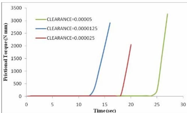
Fig. 5 Effect of Clearance on Frictional torque
