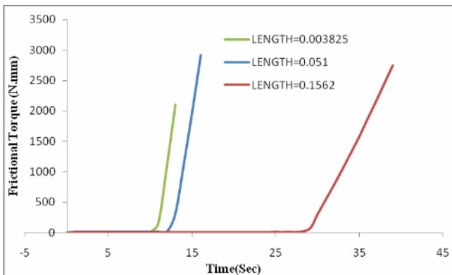
Fig. 4 Effect of bearing Length on Frictional torque
