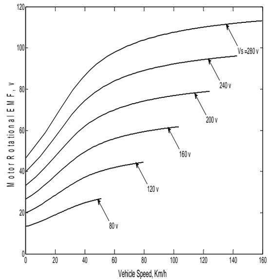
Figure 12. Motor rotational EMF versus vehicle speed during acceleration.
