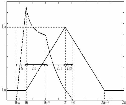
Figure 2. Motor phase inductance and current against the rotor position
