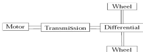
Figure 1. The EV Drivetrain
