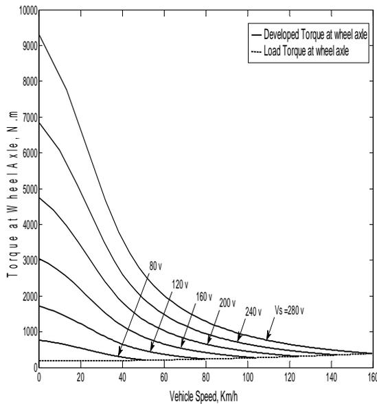
Figure 5. Torque at wheel axle versus vehicle speed during acceleration.
