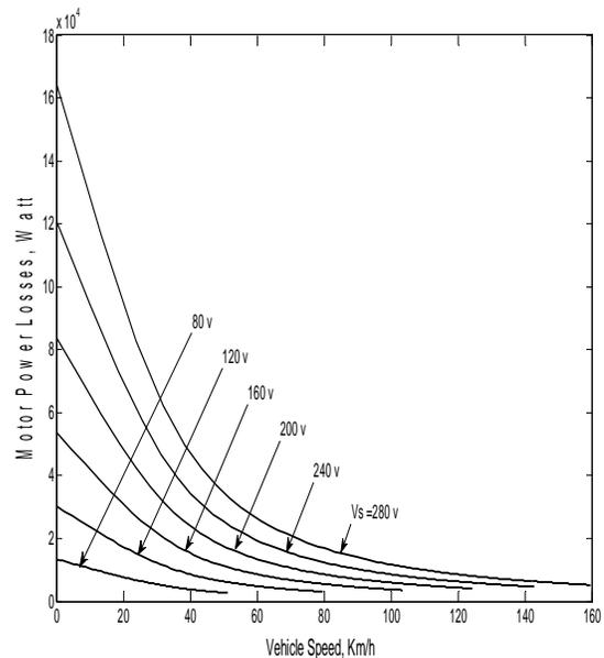
Figure 9. Motor power losses versus vehicle speed during acceleration.
