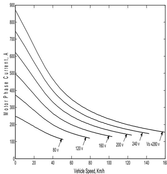
Figure 8. Motor phase current versus vehicle speed during acceleration.
