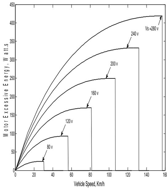
Figure 10. Motor excessive energy versus vehicle speed during acceleration.
