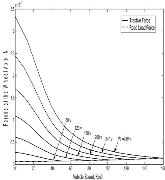
Figure 4. Tractive and resisting forces at wheel axle versus vehicle speed during acceleration.
