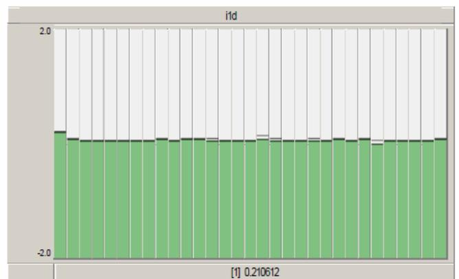
Figure 6. Current harmonic components of d axis before using active filter
