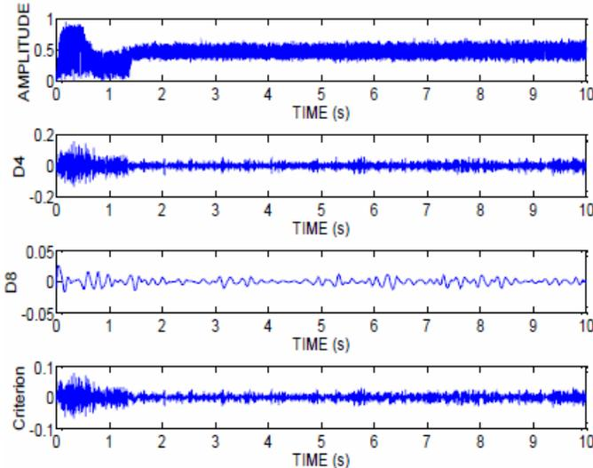
Figure 4. Voltage at PCC point and the presented criterion
