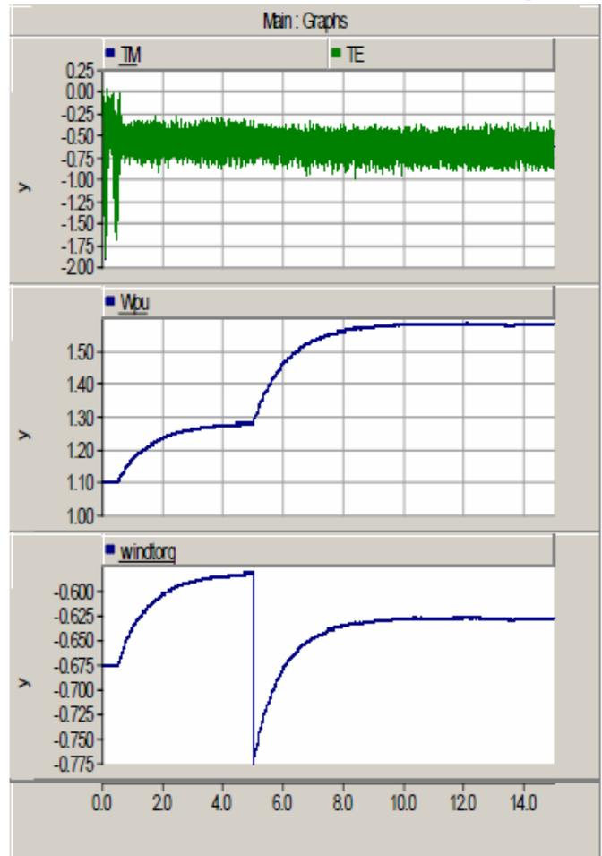
Figure 9. Controlled torques and speed after using active filter using a step disturbance at speed at 0.5 sec
