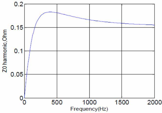
Figure 7. Frequency impedance in capacitor bus before using active filter
