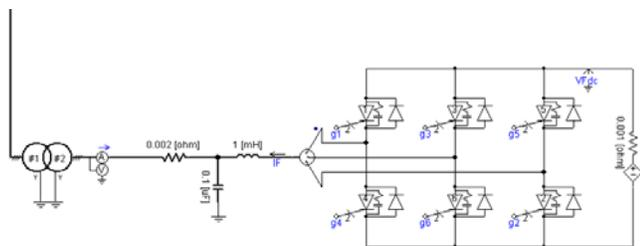
Figure 2. Three phase passive filter for series configuration
