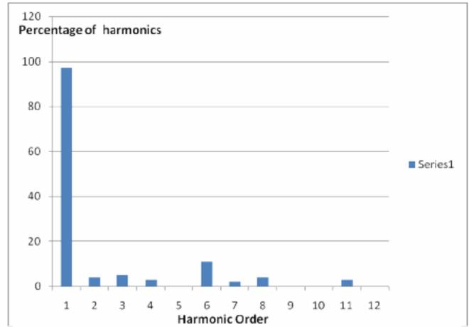
Figure 13. Voltage at PCC point energy before using active Filters
