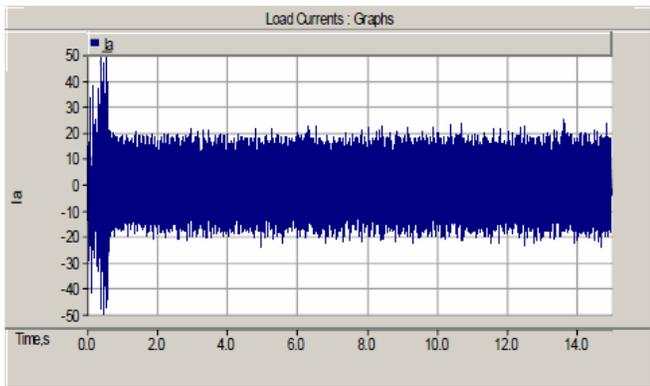
Figure 8. Current of load phase a after using active filter
