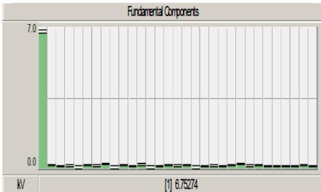
Figure 10. Current harmonic components after using active filter
