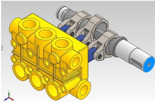
Fig.2. 3D model of the pump
