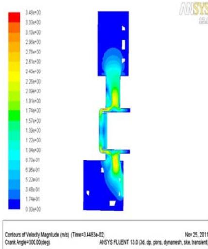
Fig. 5: Contour of velocity magnitude
