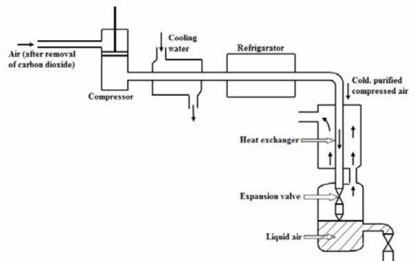
Figure-2 Liquefaction of air by Joule-Thompson cooling effect
