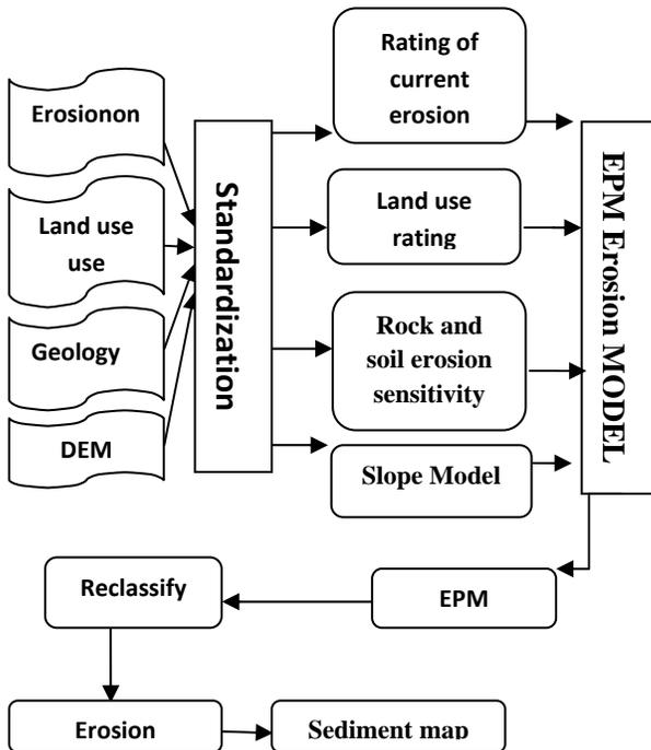
Figure 2: Processing in EPM model
