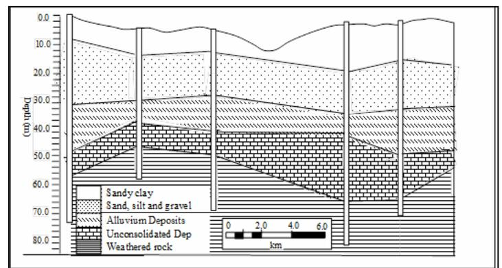
Figure 3. A geological cross section of the site
