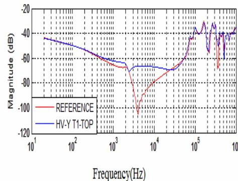
Figure 7. Magnitude responses of reference and inter-turn deformation faults of HV-Y.
