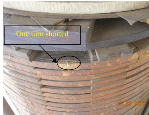
Figure 6. A view of test specimen with inter turn deformation at top position of HV-Y limb
