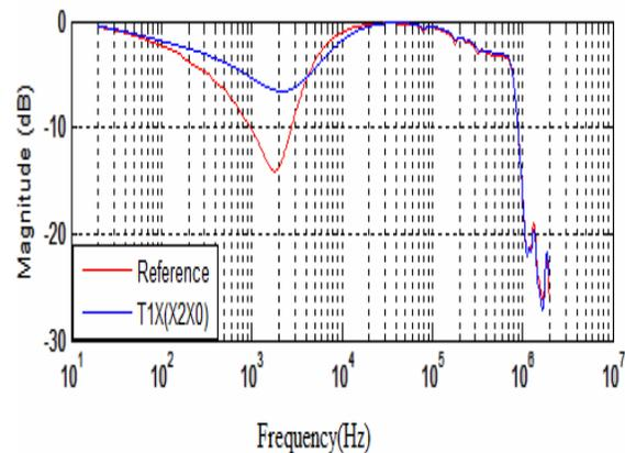
Figure 8. Magnitude responses of reference and inter-turn deformation faults of LV-y.
