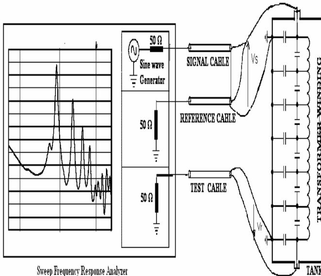
Figure 2. Schematic of the experimental set up for SFRA measurements.
