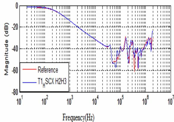
Figure 9. Magnitude responses of reference and inter-turn deformation faults of HSCX-Y.
