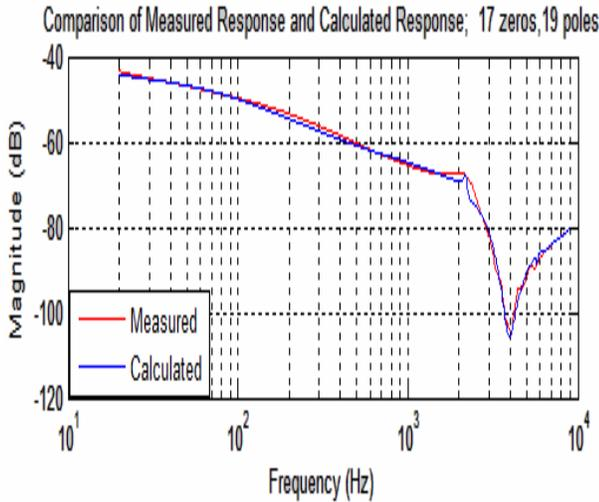
Figure 5. Measured and calculated magnitude response of transformer winding.
