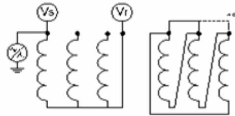
Figure 4. End-to-end (short-circuit) measurements
