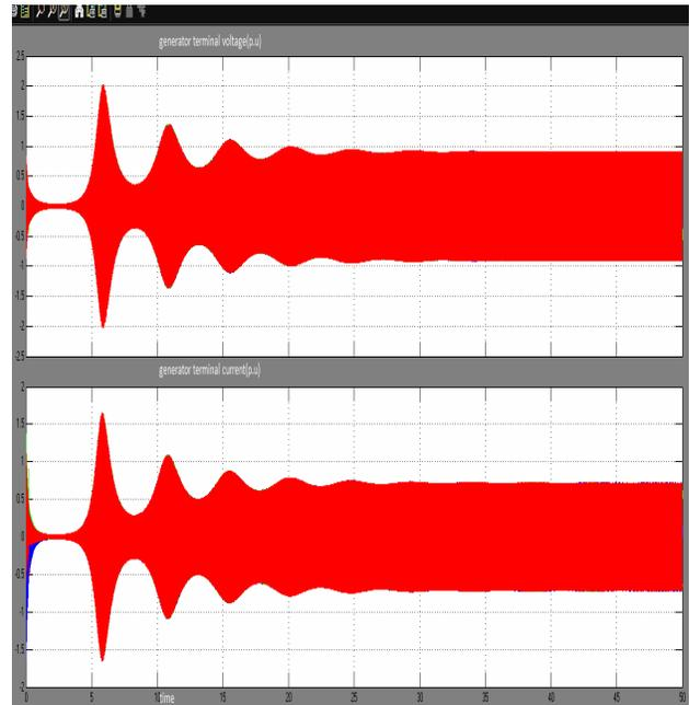
Fig.14 induction generator terminal Voltage  $V_L$ , and line Current  $I_L$
