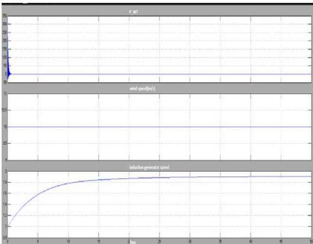
Fig.3 Power in KW, wind speed in m/s and induction generator speed in p.u.
