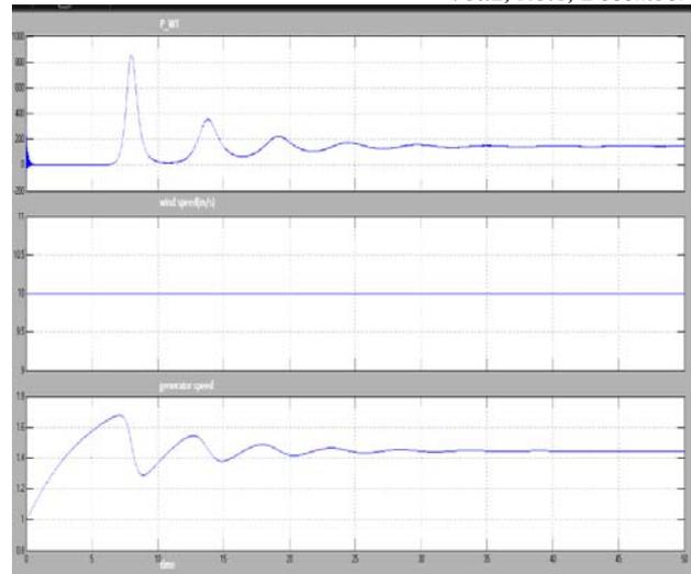
Fig.13 Power in KW, wind speed in m/s and induction generator speed in p.u.
