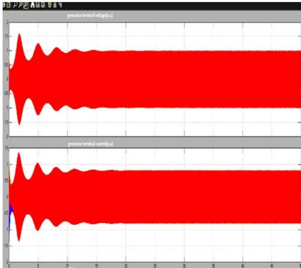
Fig.16 induction generator terminal Voltage  $V_L$ , and line Current  $I_L$
