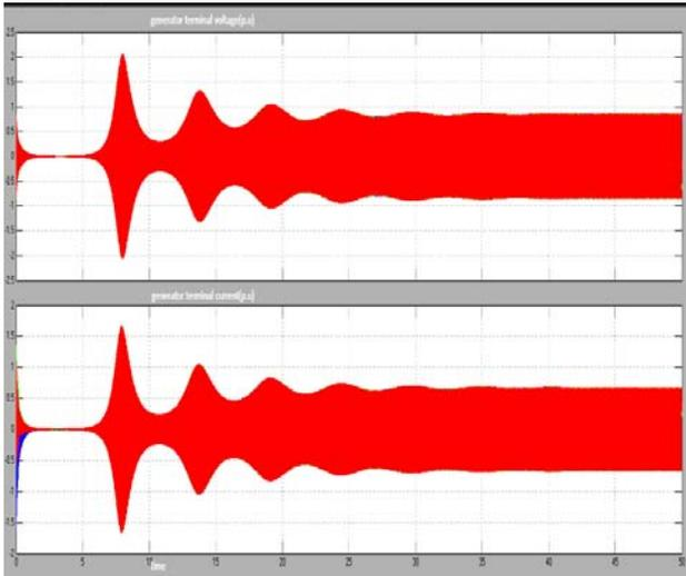
Fig.12 induction generator terminal Voltage  $V_L$ , and line Current  $I_L$
