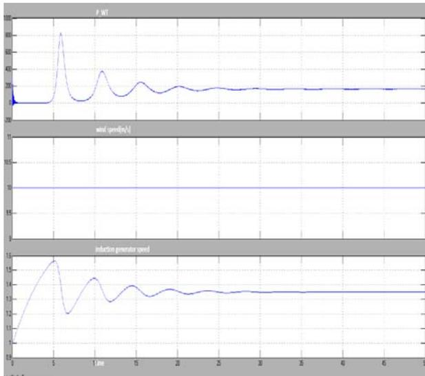
Fig.15 Power in KW, wind speed in m/s and induction generator speed in p.u
