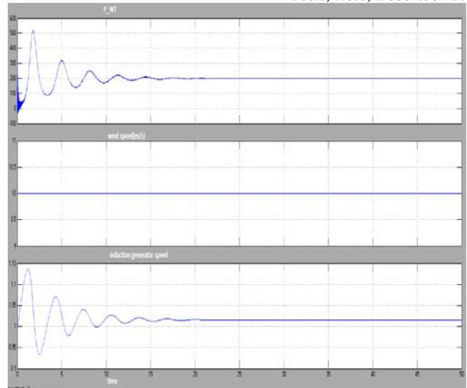
Fig.17 Power in KW, wind speed in m/s and induction generator speed in p.u.
