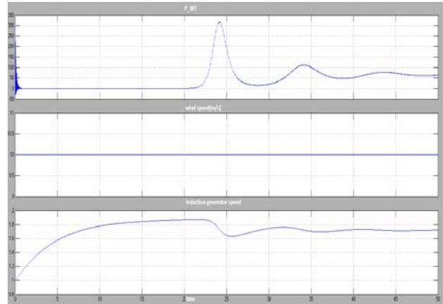
Fig.9 Power in KW, wind speed in m/s and induction generator speed in p.u.
