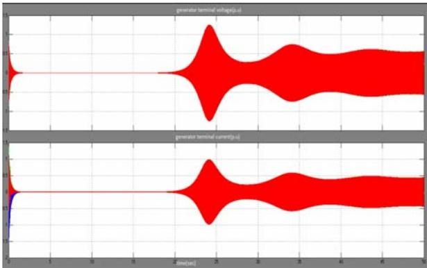
Fig.8 induction generator terminal Voltage  $V_L$ , line Current  $I_L$
