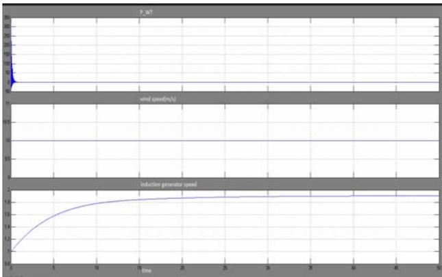
Fig.7 Power in KW, wind speed in m/s and induction generator speed in p.u.
