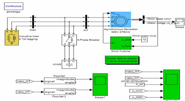
Fig.18 Simulink Model
