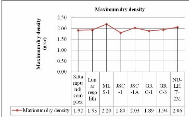
Fig.6 Maximum Dry Density Of Various Simulants
