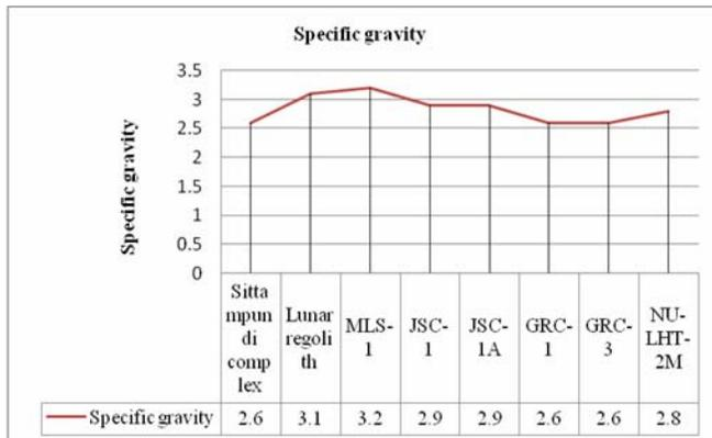
Fig.2 Specific Gravity of various Simulants
