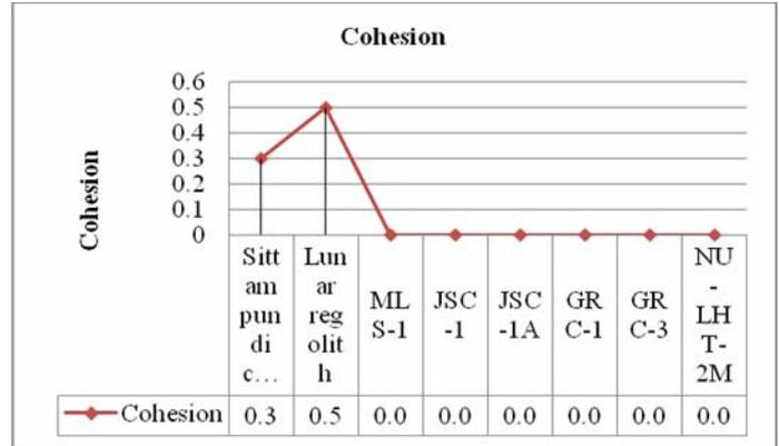
Fig.3 Cohesion value of various Simulants
