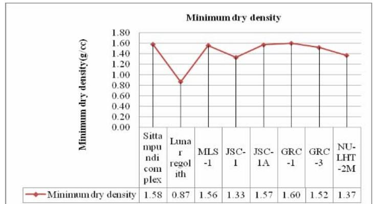
Fig.5 Minimum dry density of various Simulants
