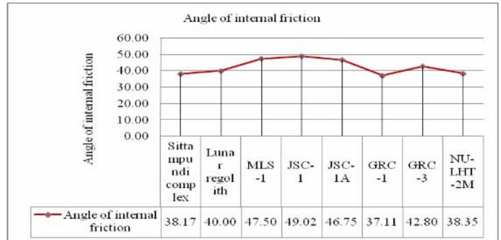
Fig.4 Angle of internal friction of various Simulants
