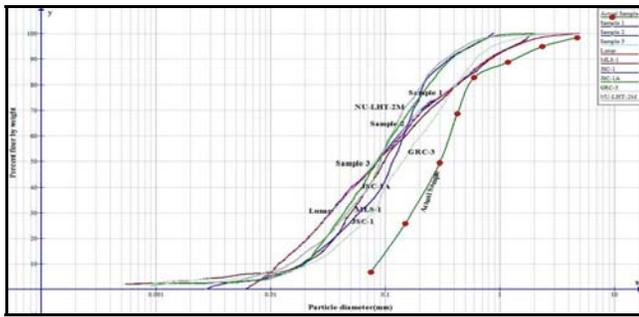
Fig.1 Grain size distribution of various simulants
