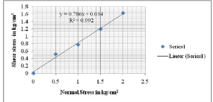
Fig.8 Shear Stress (kg/cm<sup>2</sup>)(Y) Vs. Normal Stress(X) (kg/cm<sup>2</sup>)
