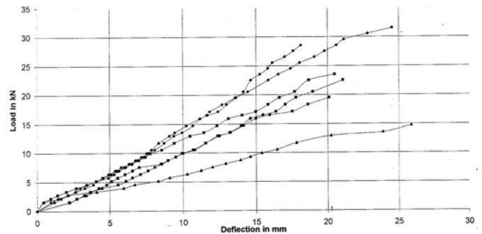
Figure 6: Comparison of Load vs Actual Deflection at Mid Span for Various Specimens
