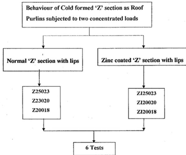
Figure 4: Details of Specimens Tested
