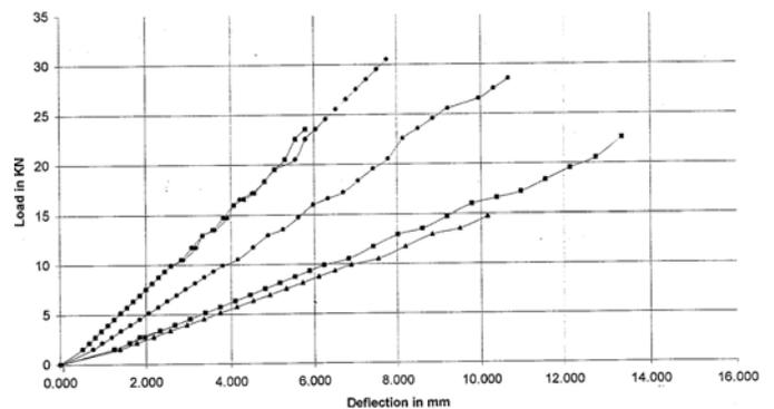
Figure 7: Comparison of Theoretical Deflection at Mid Span for Various Specimens
