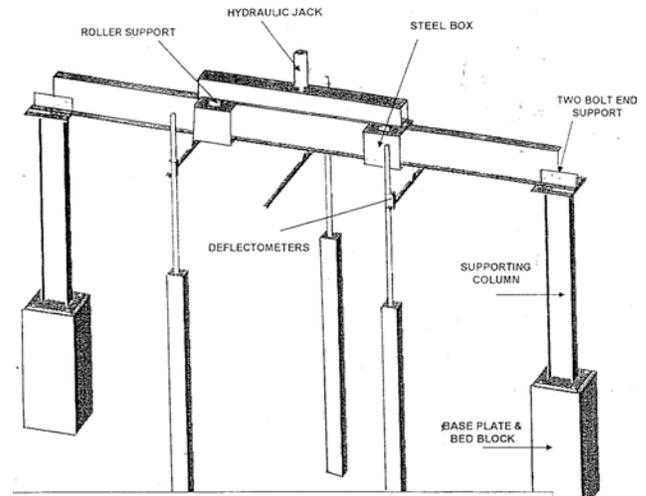
Figure 3: Schematic Diagram of Loading Setup
