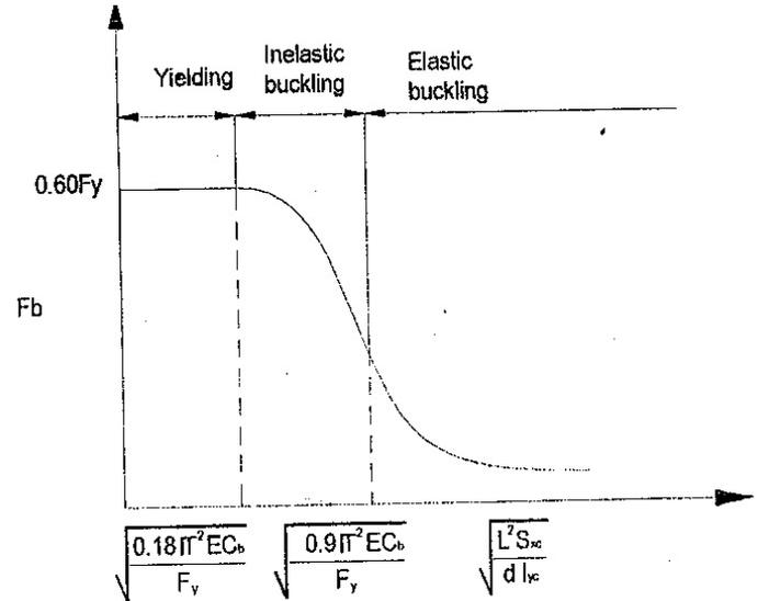
Figure 1: Allowable Stress for lateral Buckling of Z-Shaped Beams
