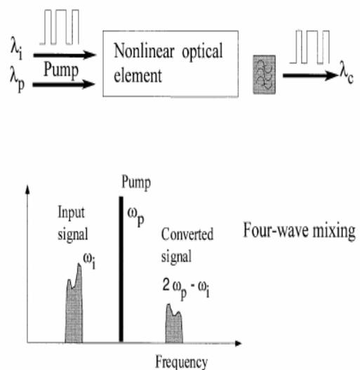
Fig. 3.3:- Schematic of conversion in nonlinear element using four-wave mixing.
