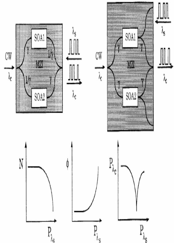
Fig. 3.4.2. Schematic and principle of operation for interferometric wavelength converters based on XPM in SOA's. (a) Asymmetric
