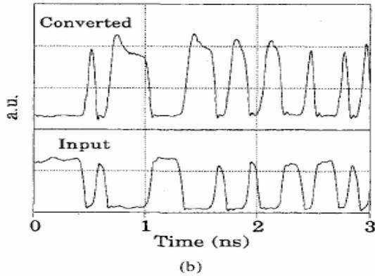
Fig. 3.4.1. Schematic of the CO- and counter-propagation XGM wavelength conversion principle (a) and measured waveforms for the converted signal (co-propagation) and the input signal at 10 Gb/s (b). The measurements are performed with a 1200 pm long SOA.
