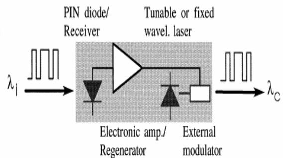
Fig. 3.1:- Schematic of opto-electronic converter.
