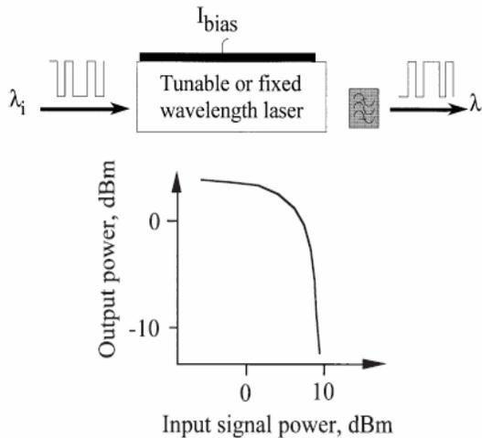
Fig.3.2:-Principle of wavelength converters based on semiconductor lasers together with schematic of output versus input power characteristic for laser converter.
