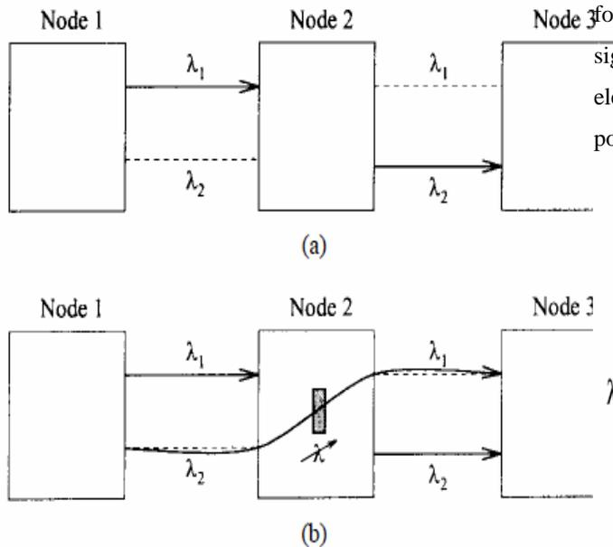
Fig. 2. Wavelength-continuity constraint in a wavelength-routed network: (a) without converter and (b) with converter.
