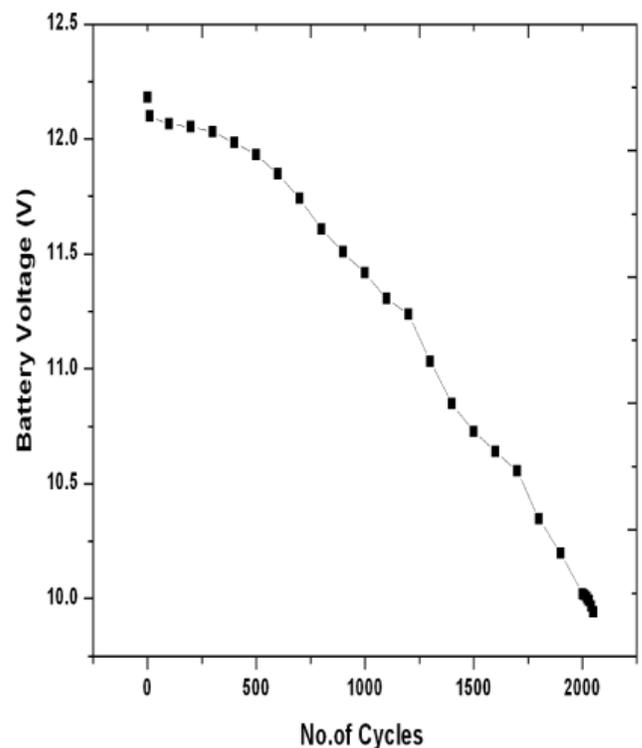
**Figure 3.** Life Cycle Analysis of 12V/17Ah Lead-Acid battery up to end of life
