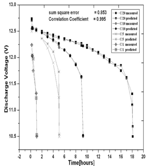
**Figure 4.** Comparison between experimental and predicted discharge curves at discharge rates of C/20, C/10, C/5, and C/1.
