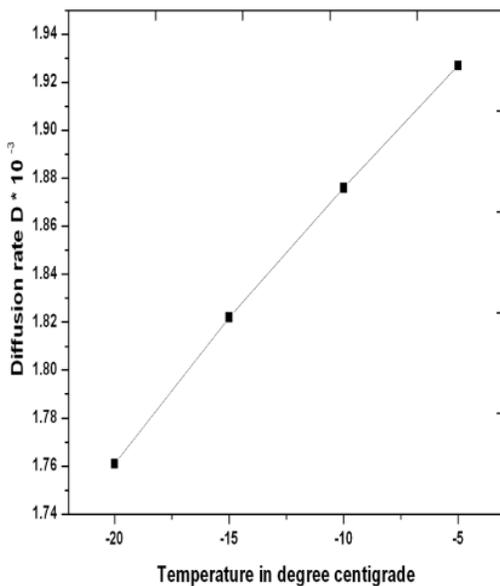
Figure 6. Diffusion rate at low temperatures
