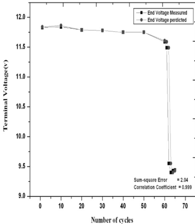
**Figure 2.** Comparison of measured and predicted data of Battery voltage Vs no.of.cycles.
