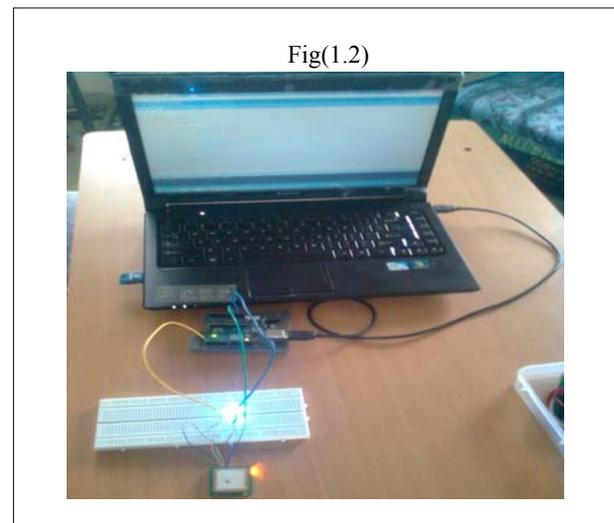
GPS-634R" is a highly integrated smart GPS module with a ceramic GPS patch antenna. The antenna is connected to the module via an LNA. The module is with 51 channel acquisition engine and 14 channel track engine, which be
