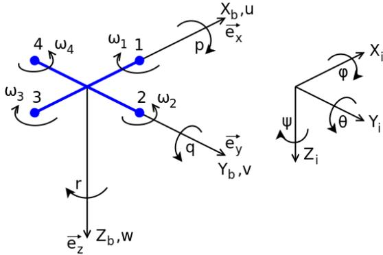
Fig.1. Quadrotor frame of reference
