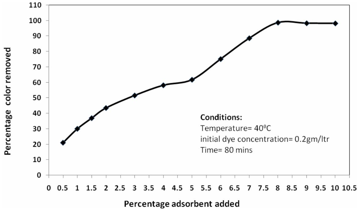
**Figure-1 Effect of amount of adsorbent addition on percentage color removal**
