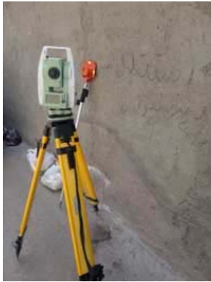
Fig.3 overview of topography camera Leica series of total Station TS02
