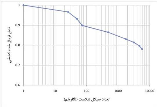
Fig.5 S-N curve of composite material under tension loading with R=0.1 based on Finite element analysis
