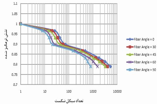
Fig.12 S-N curve of unidirectional composite with different fiber angles under axial tension loading
