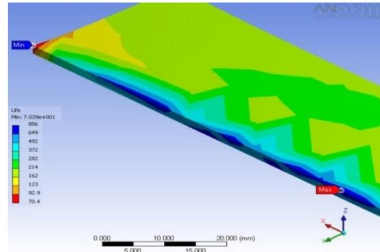
Fig.16 Fatigue life contour of composite under axial tension load in the transverse direction
