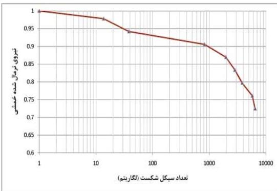
Fig.11 S-N curve of composite material under three point bending fatigue
