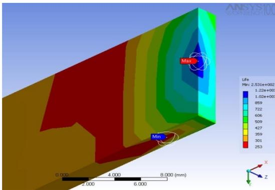
Fig.14 Fatigue life contour of composite under axial tension load in the fiber direction
