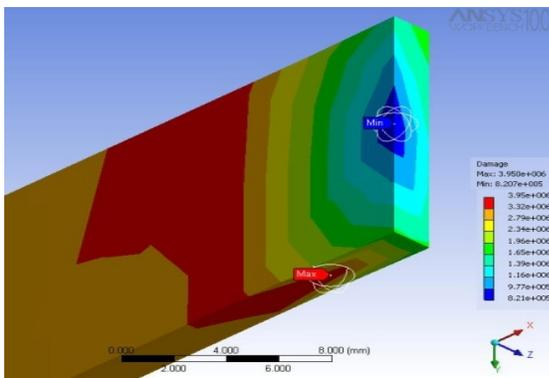
Fig.15 Fatigue damage contour of composite under axial tension loading in the fiber direction
