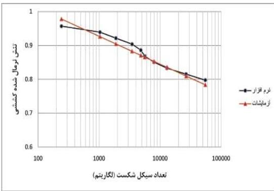
Fig. 2 S-N curve of matrix under tension loading with R=0.1
