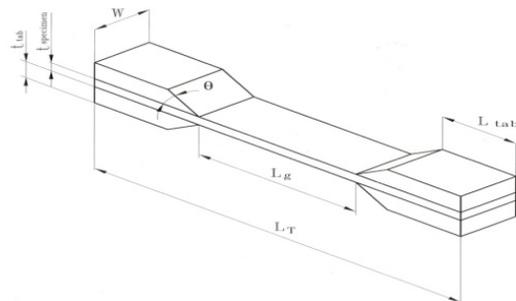
Fig.4 Experimental geometry of the longitudinal properties of composite [13]
