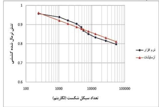
Fig. 3 S-N curve of fiber under tension loading with R=0.1
