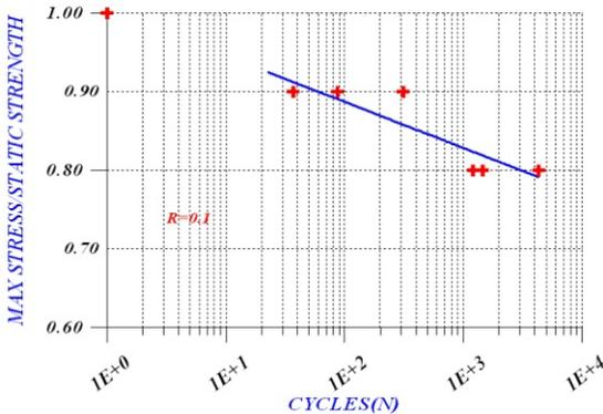
Fig.6 S-N curve of composite material under tension loading with R=0.1 based on experimental data [6]
