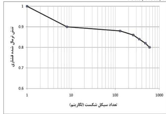
Fig.7 S-N curve of composite material under tension loading in the transverse direction with R=0.1 based on Finite element analysis
