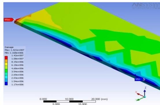
Fig.17 Fatigue damage contour of composite under axial tension load in the transverse direction
