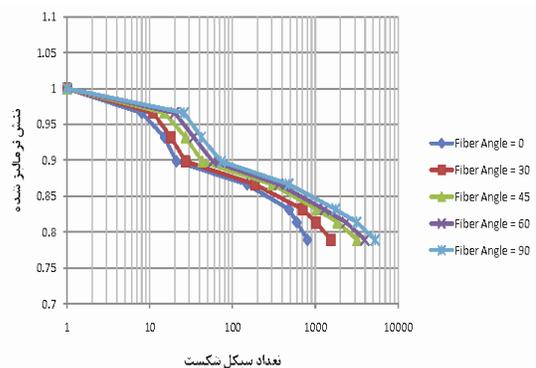
Fig.13 curve of unidirectional composite with different fiber angles under axial compression loading
