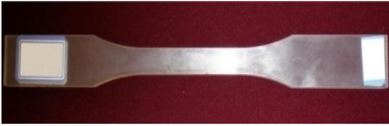
Fig. 1 Experimental specimen [7]
