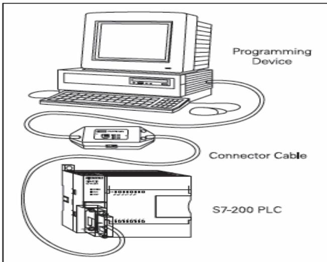
Figure 4. Configuration of PLC with computer
