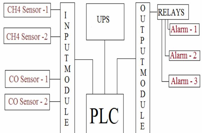
Figure 6. Block diagram of automatic gas monitoring and power cut-off system
