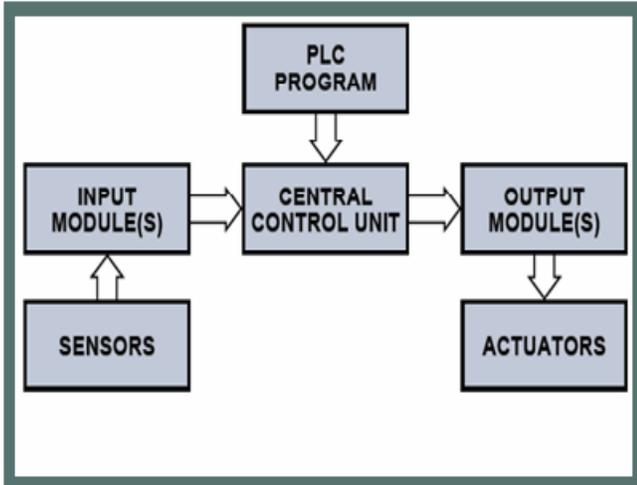
Figure 3. Basic operation of PLC system
