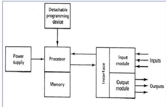
Figure 2. Architecture of PLC
