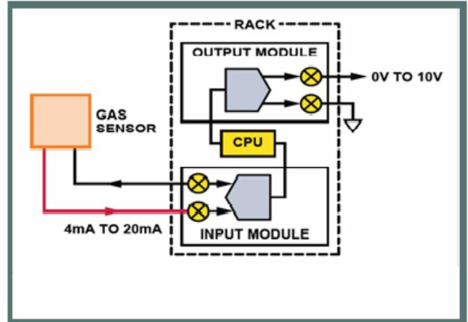
Figure 5. Gas sensing system
