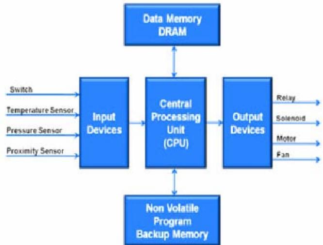
Figure 1. Block diagram of PLC
