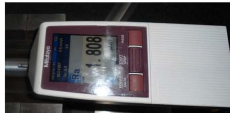
**Figure- 2 Surface roughness Tester SJ-210**
