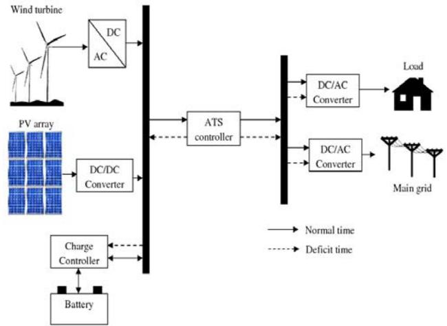
Figure 1. PV/Wind/Battery Hybrid System Configuration.
