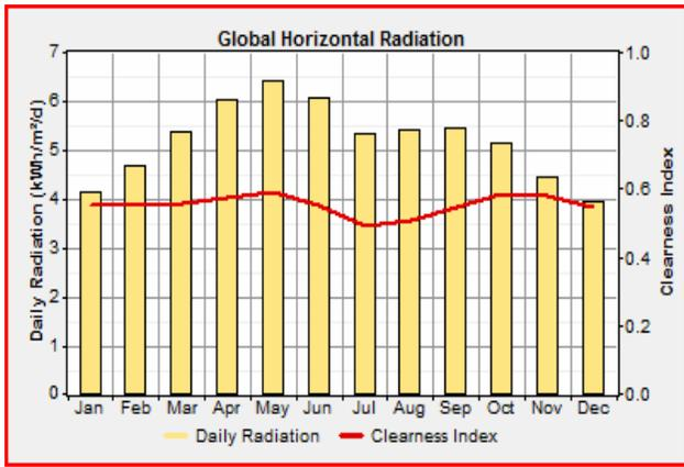
Figure 2. Solar radiation of Oman.
