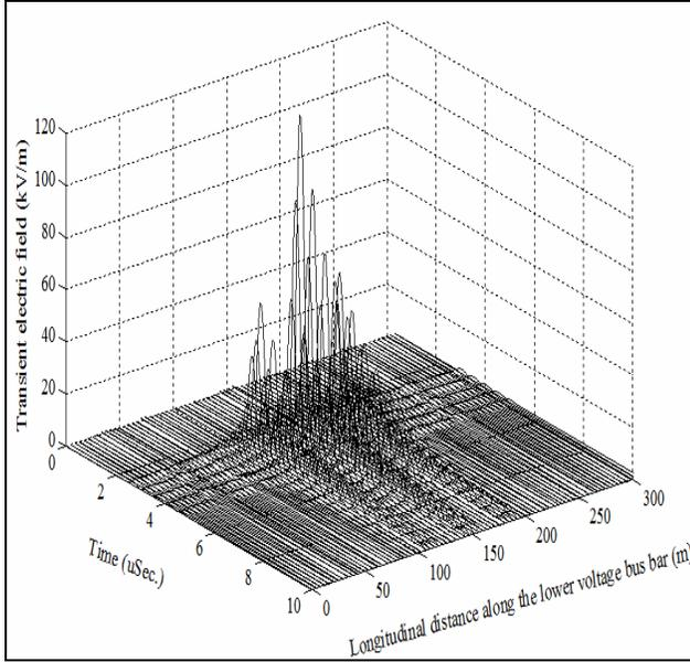
Fig.9. Variation of transient electric field (kV/m) along the lower voltage bus bar with switching line L3
