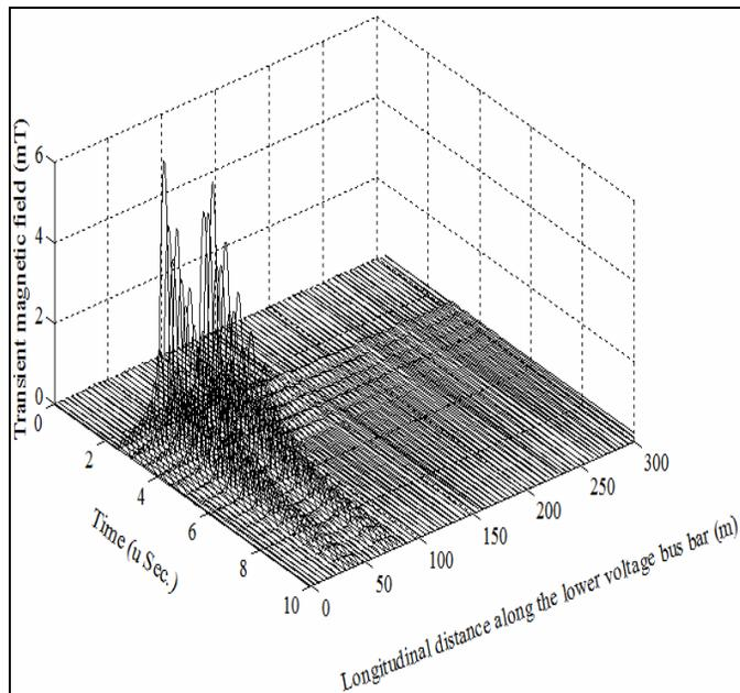
Fig.5. Variation of transient magnetic field ( $\mu$ T) along the lower voltage bus bar with switching line L1
