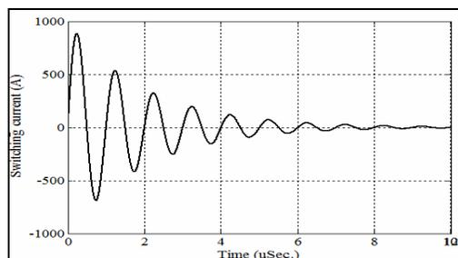
Fig.3: Transient sinusoidal switching current (A).
