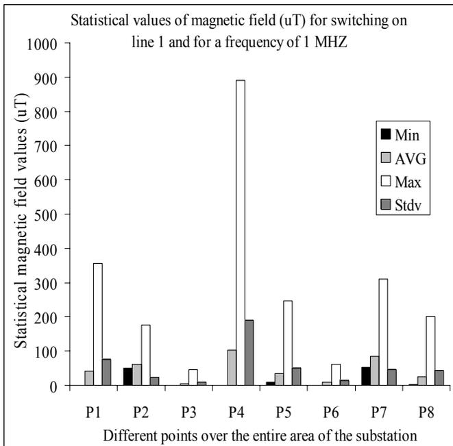
Fig. 7. Statistical transient magnetic field values ( $\mu\text{T}$ ) at different points for switching on line 1 with frequency of 1 MHz.
