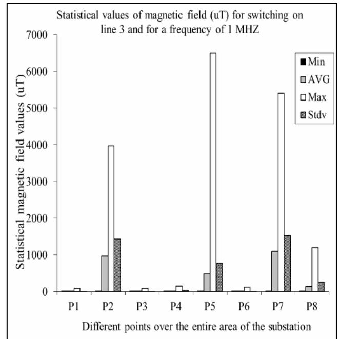
Fig. 8. Statistical of transient magnetic field values ( $\mu\text{T}$ ) at different points for switching on line 3 with frequency of 1 MHz.
