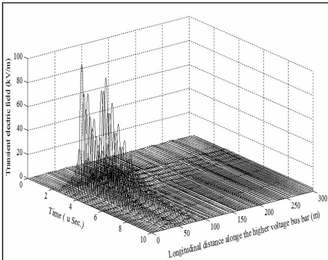
Fig.10. Variation of transient electric field (kV/m) along the lower voltage bus bar with switching line 1.
