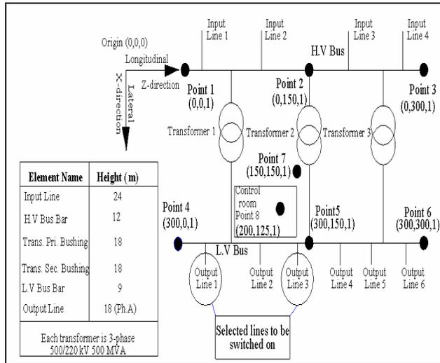
Fig. 1. Simple layout of the substation 500/220 kV.
