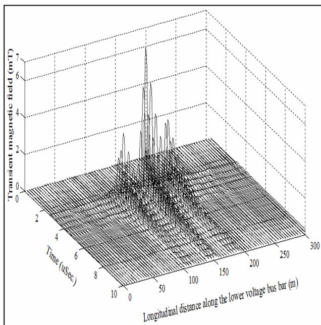
Fig.4. Variation of transient magnetic field ( $\mu$ T) along the lower voltage bus bar with switching line L3
