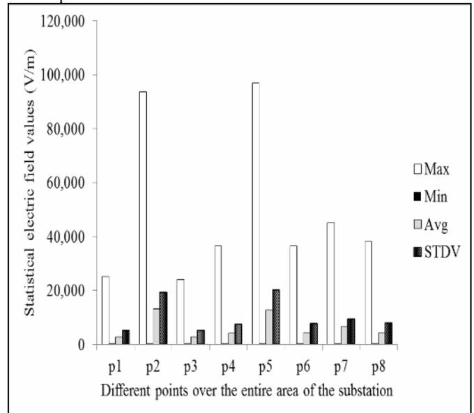
Fig. 12. Statistical of transient electric field values (V/m) at different points for switching on line 3 with frequency of 1 MHz.
