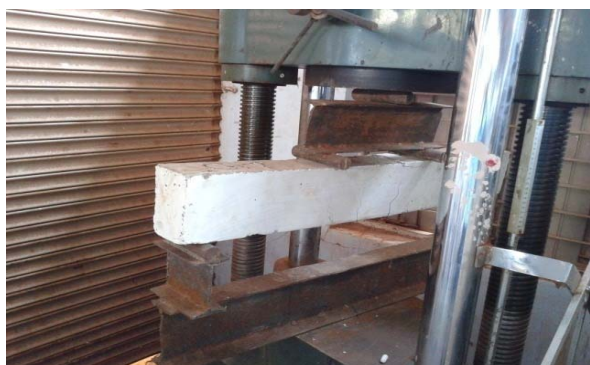
Figure 6. Flexure test on RCC beam- Experimental setup
