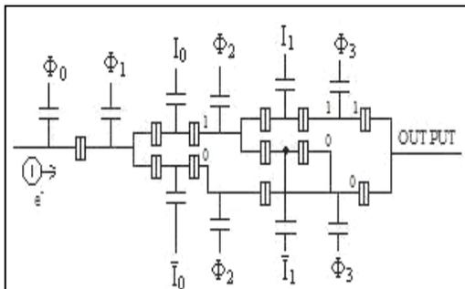
Figure 5. 2 input AND Gate using SET
