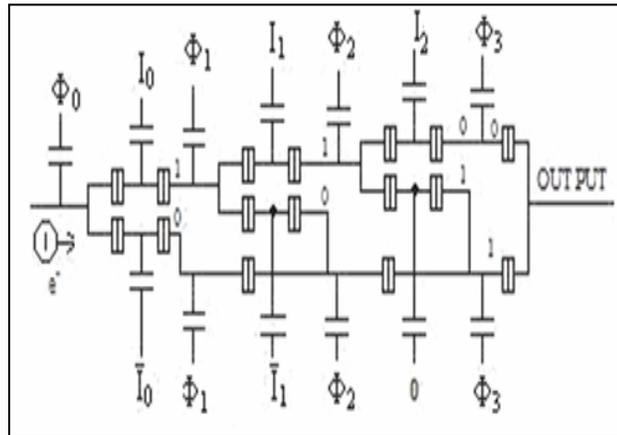
Figure 9. 2 input NAND Gate using SET
