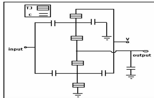
Figure 7. 2 input NOT Gate using SET
