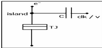
Figure 3. Passing of electrons in Tunnel Junction
