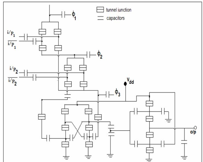
Figure 8. 2 input NOR Gate using SET
