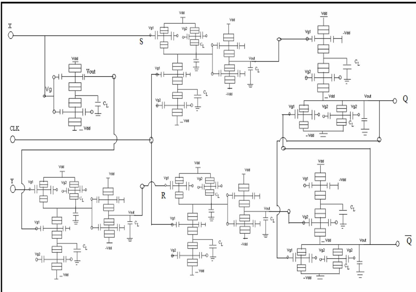
Figure 10. SET Logic Gate Based Level Sensitive SR Latch IC
