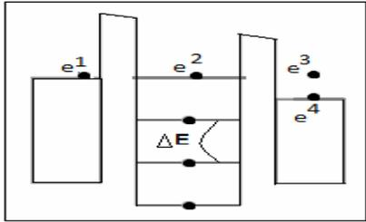
Figure 2. Energy Levels of the Island Electrode Coulomb Blockade
