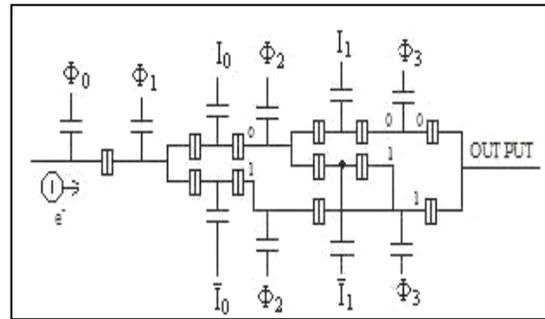
Figure 6. 2 input OR Gate using SET
