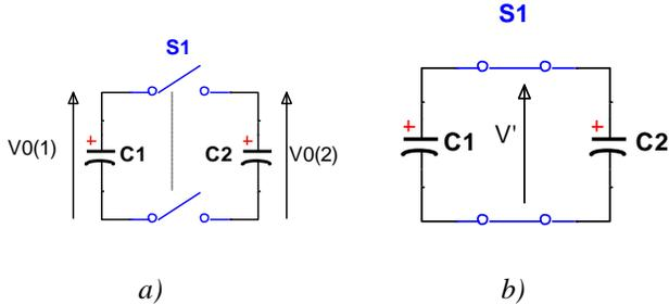
Figure 1. Charge transfert circuit
