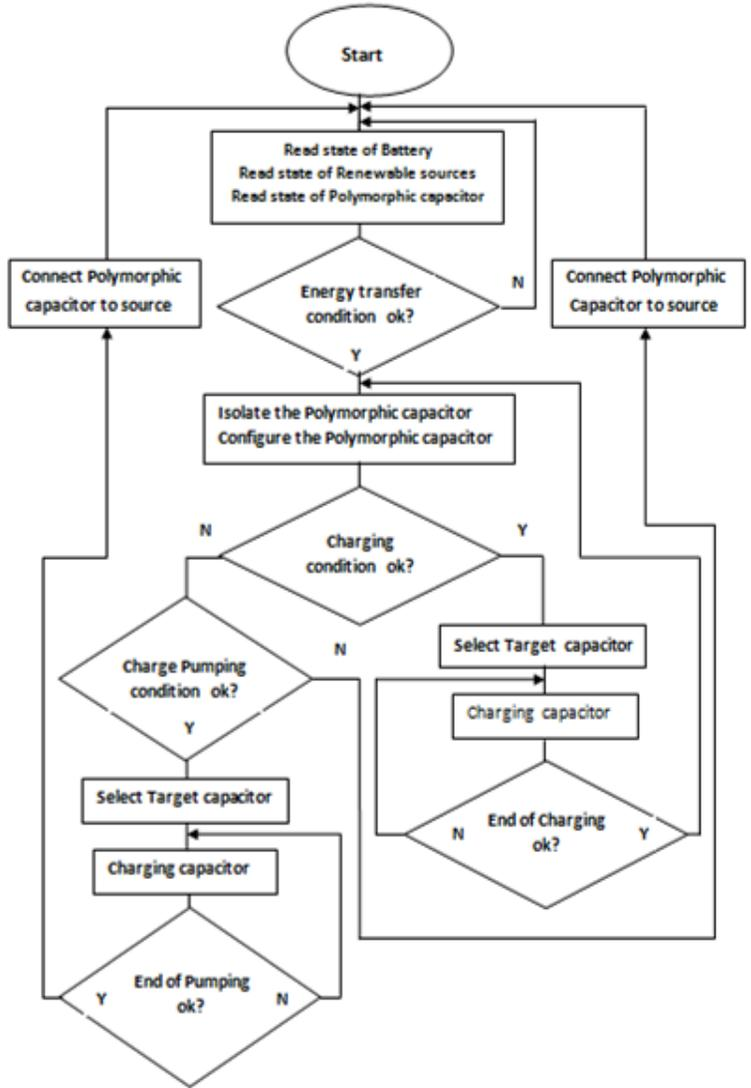
Figure 8. Polymorphic capacitor storage algorithm
