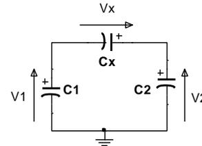
Figure 5. The pump charge circuit using Polymorphic capacitor  $C_x$
