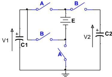
Figure 3. Example of a pump of charge circuit
