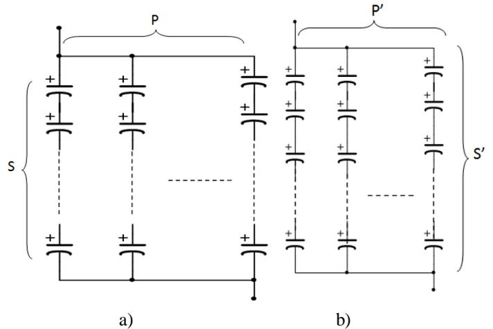
Figure 6. a polymorphic switched capacitor structure.
