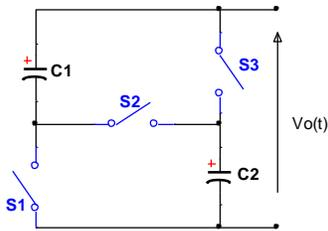
Figure 7. Elementary cell for serial /parallel capacitors association
