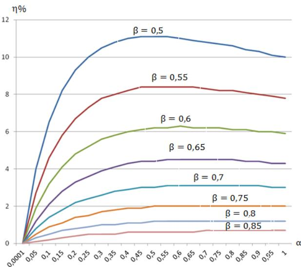
Figure 2. Variation of the energy loss ratio η=f(α, β)
