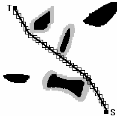
Figure 6. The first example illustrates a path planning of a boat. Such an environment is populated by a group of islands seen as obstacles to what you can add boats supposedly immobile. The problem then is to determine the shortest path without collision from a starting point S to a point of arrival T. The obstacles are dilated by the size of the moving object (the boat in our case): the shaded area.
