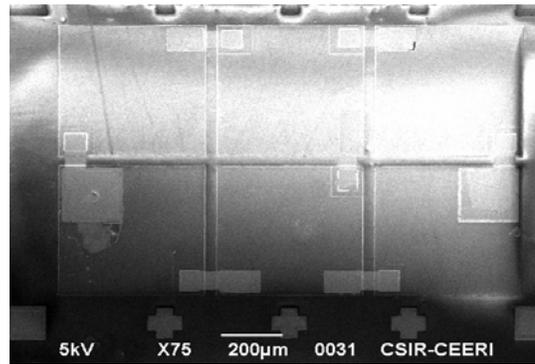
Fig. 3 SEM picture of the fabricated GaN blue alternating-current (AC) light-emitting diode.
