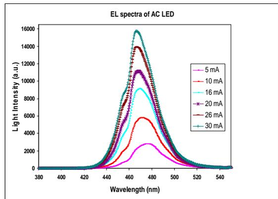
Fig. 8 Room temperature EL spectra of InGaN/GaN MQWs AC- LED at different injection current (dc).
