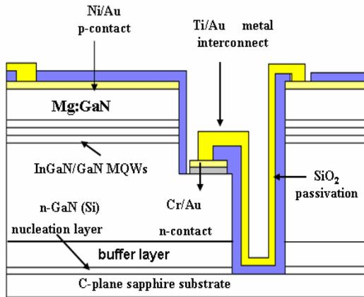
Fig. 1 Schematic structure of the GaN blue alternating-current (AC) light-emitting diode.
