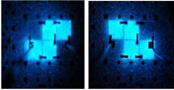
Fig. 5 Top view photographs of the AC blue LED illumination under (a) positive and (b) negative dc voltage (13V).
