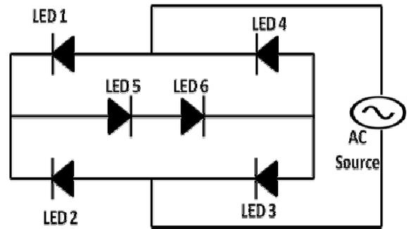
Fig. 2 Circuit diagram of Wheatstone Bridge AC-LED
