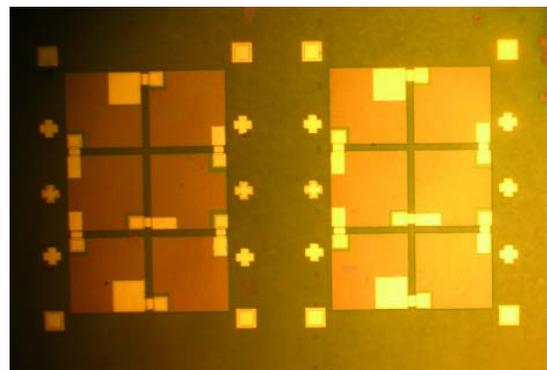
Fig. 4 Photograph of fabricated high voltage GaN AC blue LED in Wheatstone bridge configuration
