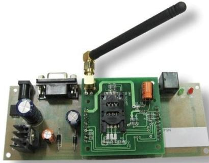
Fig.7 GSM modem: SIM 300 Modem
