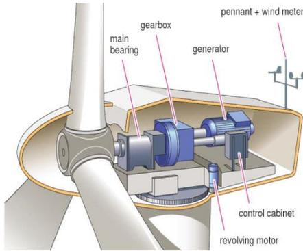
Fig2.1. Wind turbine nacelle cross-section.
