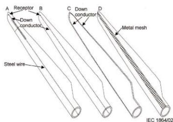
Fig.6.3. Lightning protection for large modern wind turbine blades
