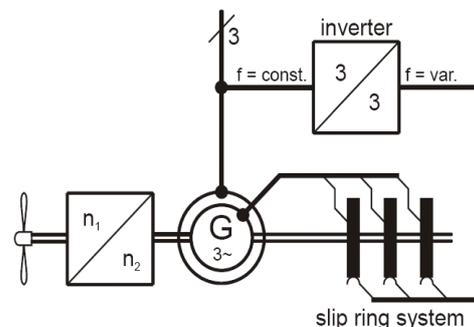
Fig.6.2.Slip ring generator system principle.
