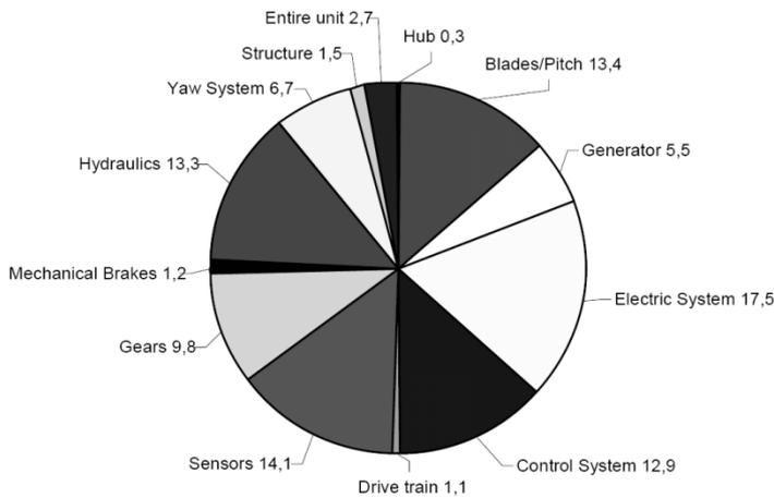
Fig.2.2. Failures number distribution [%] for Swedish wind power plants.
