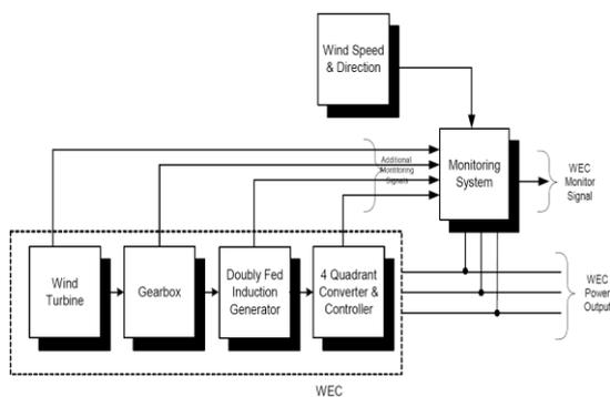
Fig.6.1. Basic architecture of WECS condition monitoring and diagnosis
