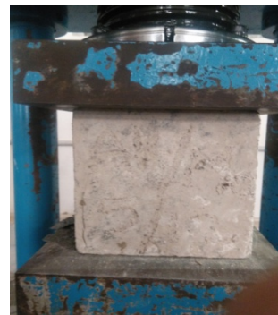
Figure 2 Compression test of concrete
