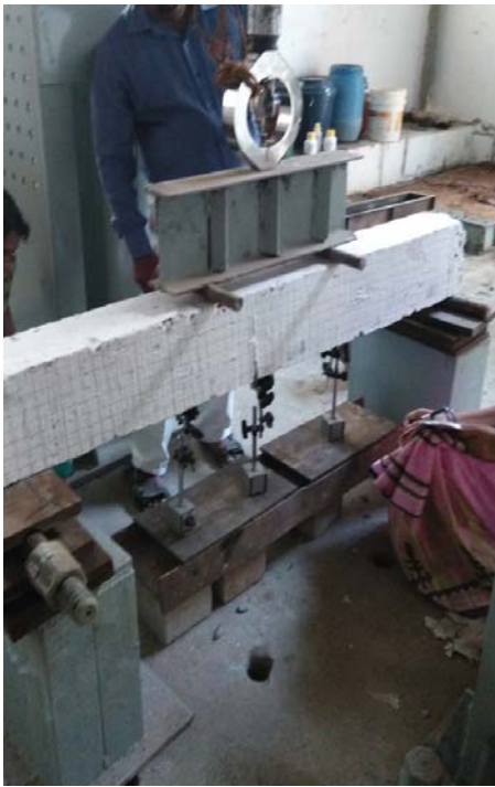
Figure 8 RCC beam set up
