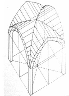
Figure 7: Structure of Kalanbeh arch, [9].
