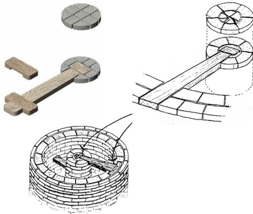
Figure 8: Connection and involvement of tensile elements (wooden beams) with the body of the minaret towers. Source: the author
