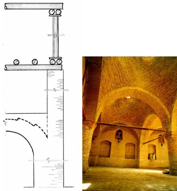
Figure 12: Using lighter material; at the bottom is the stone foundation, at the middle is the brick wall, followed by a wooden and brick roof to cope with bending [14]
