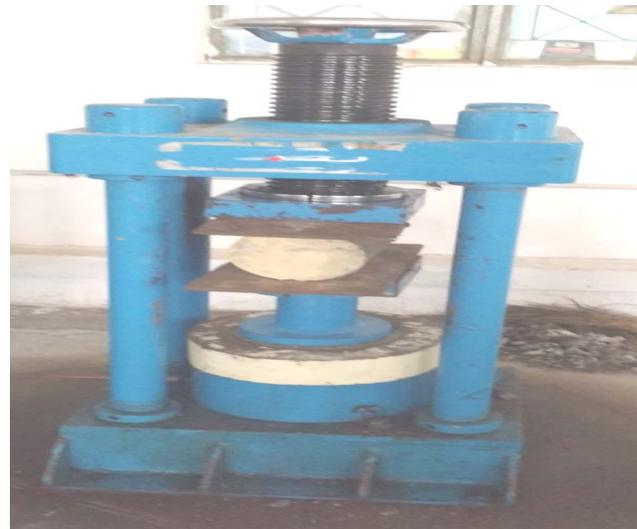
**Figure 3-Test setup for cylinder specimen**
