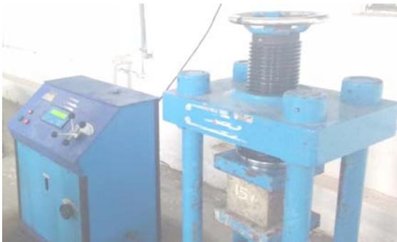
**Figure 2-Test setup for cube specimen**
