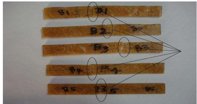
Fig. 6 Photograph of specimens after flexural fracture
