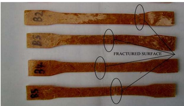
Fig. 4 Photograph of specimens after tensile fracture
