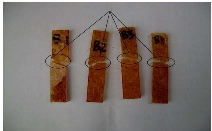
Fig. 7 Photograph of specimens after impact fracture
