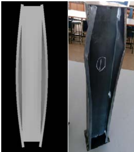
Fig.2 Failure modes with lip – Numerical Vs Experimental
