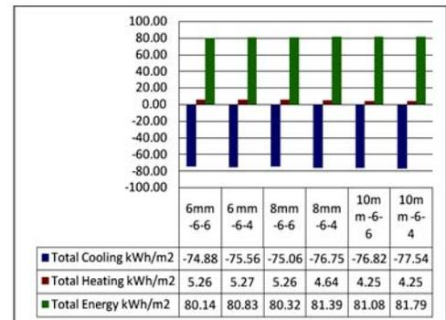
The optimum state was also obtained in this section, which due to lower annual energy consumption, the optimum state has been related to a façade in which the thickness of external glass and internal glass were respectively 6 mm and 6 mm and the distance between two glasses was 6 mm. Then, this state was simulated by simple, matt and reflective glass, which following diagram shows the energy consumption in this envelope.
