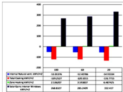
DIAGRAM 7: ENERGY CONSUMPTION FOR COOLING AND HEATING AND NATURAL VENTILATION AND SOLAR GAINS IN DOUBLE-SKIN FAÇADE WITH EXHAUST FAN CONSIDERING DIFFERENT DISTANCES BETWEEN TWO SKINS
