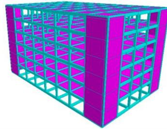
Fig 1: Shear wall at the edge
