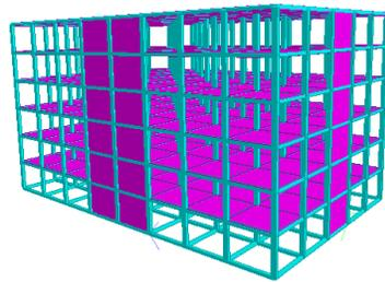
Fig 2: Shear wall at the center of each side
